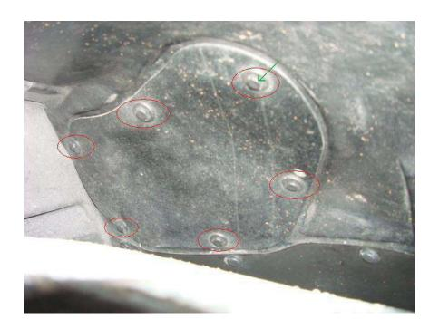
3) Rivets removed and back of housing exposed. The yellow box (below) denotes the location of the DRLs/turn signals in this case, for those just twist and remove, bulb and bulb housing right there (See below). Re-install and you're done.
